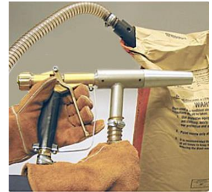
Gun with Suction Tube in bag of abrasive
